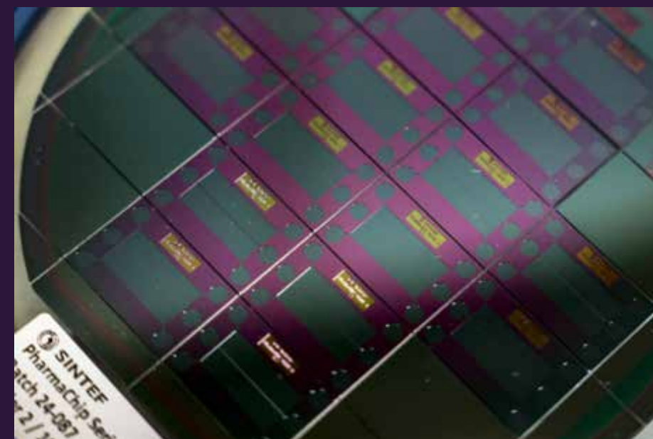
Figure 1. Zoom-out of electroextraction chips which are manufactured in a scalable and reproducible fashion using micro- and nanofabrication technology. The design has been submitted as a patent application.
