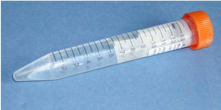
Figure 6.1: Mouse load phantom. Trap the air bubble at the top position of the phantom.
