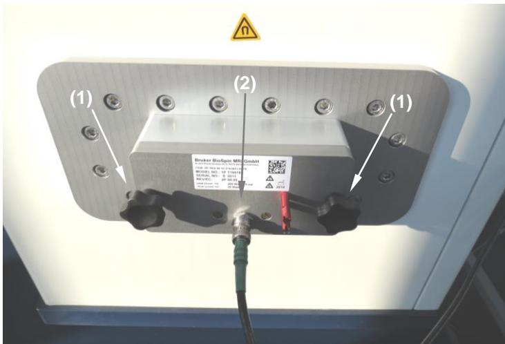
Figure 5.9: RF Coil connection located on the rear side
