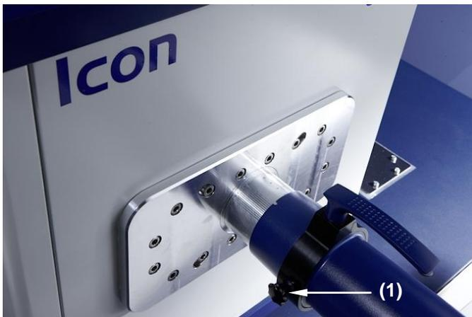
Figure 2.8: The animal holder was inserted into the magnet and locked in place with knurled screw (1)
