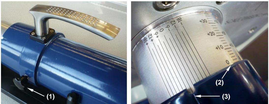
Figure 5.14: Fixate the Basic Animal Holder in the magnet with the knurled screw (1). Two scales, one for horizontal shifts (2, with 2-mm division), and one for rotation (3, with 3-degree division) facilitate positioning. The Magnet Center Position is reached when both scales show zero.
