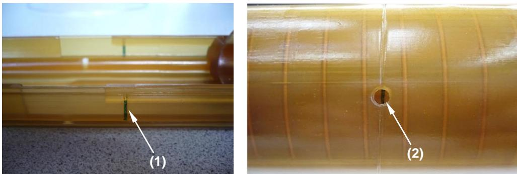
Figure 5.12: (1) Magnet Center marking on the animal bed. (2) The hole in the body RF Coil was aligned with the Magnet Center marking.
