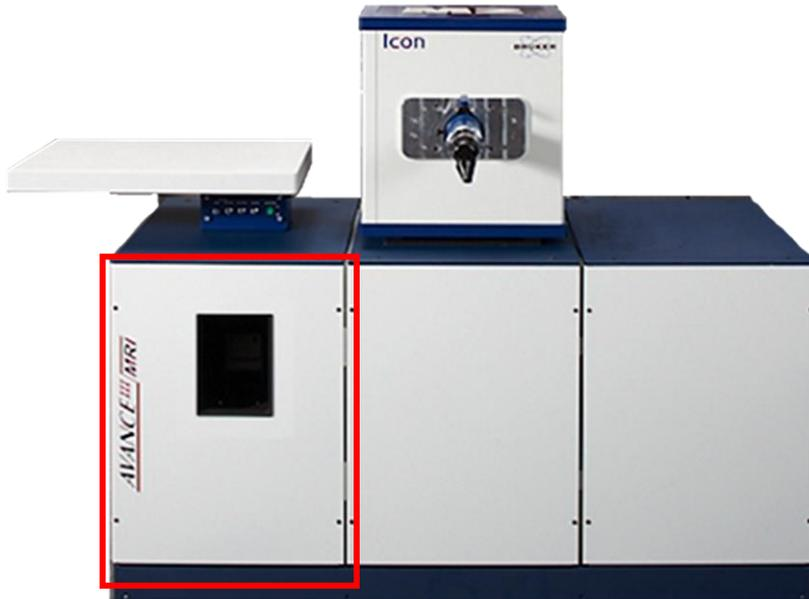
Figure 2.4: The left-most cabinet is prepared for the usage of an anesthetic gas evaporator and an anesthetic scavenging system.
