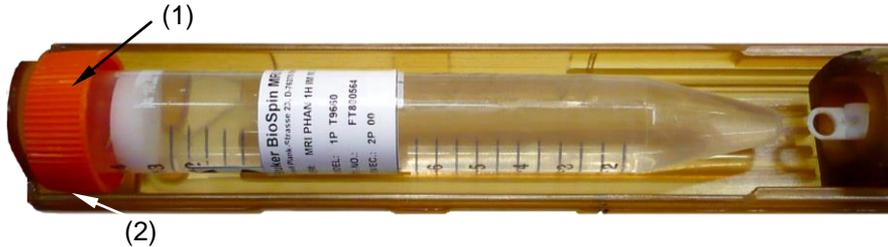
Figure 6.3: Placement of the mouse load phantom on the mouse body animal bed. The cap (1) of the phantom rests in the deepening (2) at the end of the animal bed. No phantom holder is needed.
