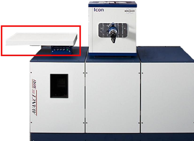
Figure 2.5: The animal preparation table provides working space and accommodates the animal holder while not in use.
