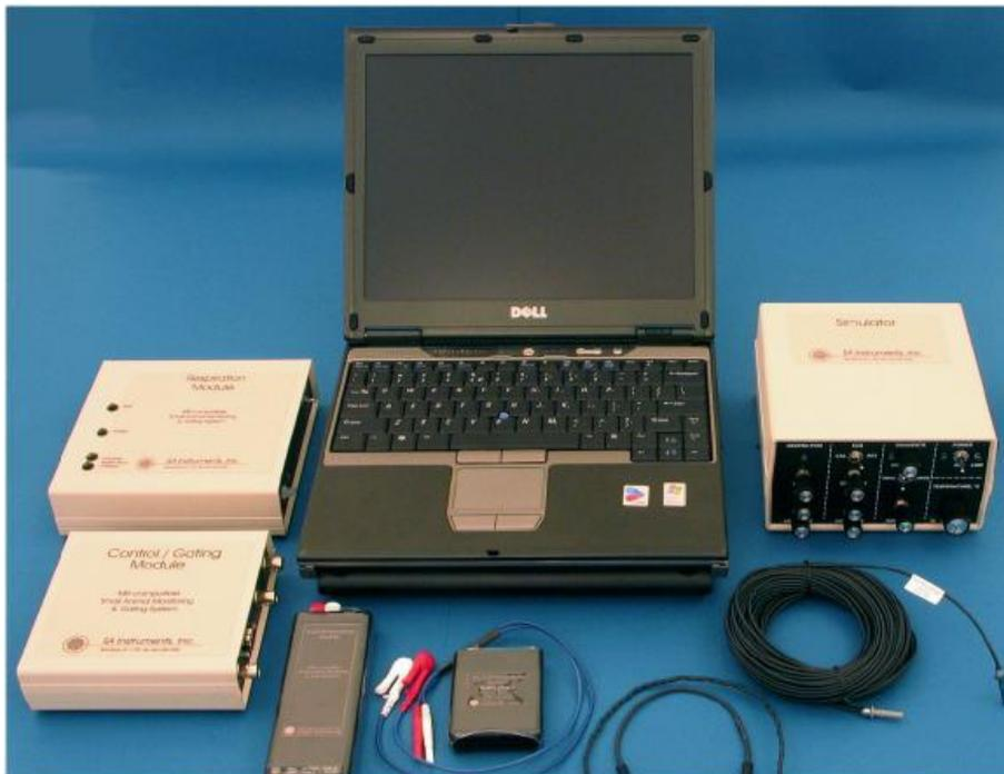
Figure 7.1: MR compatible small animal monitoring and gating system (option)
