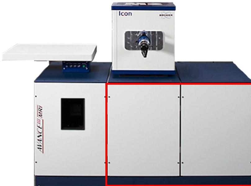
Figure 2.3: The red marked cabinets contain all electronic components. No user interference is needed within these cabinets.
