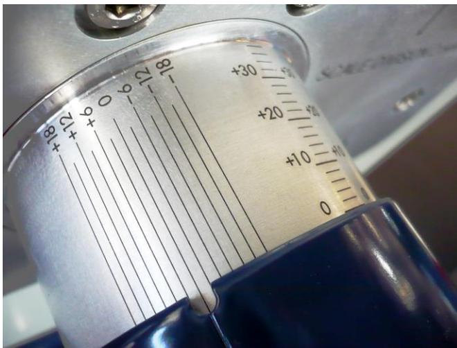
Figure 2.9: The position and rotation of the animal holder with respect to the magnet center may be read from the magnet front flange.
