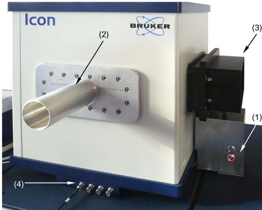
Figure 2.2: ICON permanent 1 T magnet. The main system switch for electronics (1) is located on the right side of the magnet. Animals or placed in the magnet through the front flange (2). The magnet has air-cooling fans on both sides (3, left fan not visible). RF Coils are attached at the connector panel (4).
