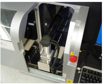
Adapter with FMT Mouse Imaging Cassette mounted in the Quantum GX2 microCT Imaging System scanner
